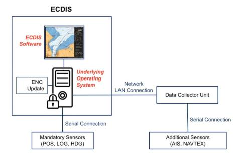
Figure 2 Architecture of the shipboard ECDIS.
